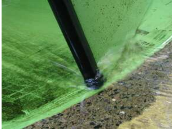
Rubber extrusion (fish bumper) after fitting
